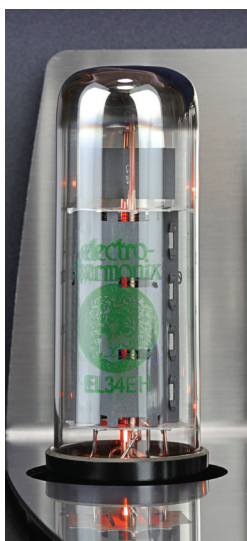
An Electro-Harmonix EL34EH power output tube, one of four.
